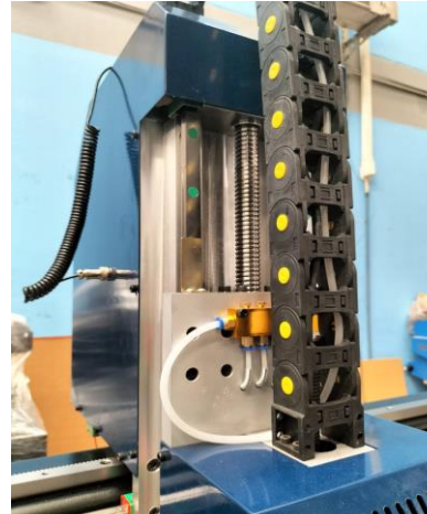
Z-core head set /ball screw up-down/ Oil Dispenser / Keel Clamp Head Z Core
