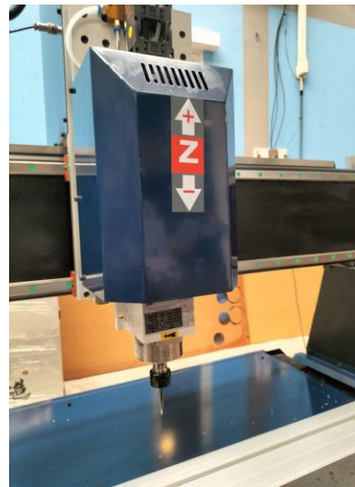
Z-axis heads that can be raised up to 330 cm high.
