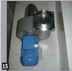
15 Air cooling extractor
