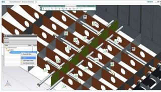
NX Platform Design provides tools to efficiently create secondary steel structure used in outfitting.
