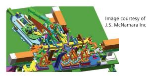
Welding fixture complete with clamps and welding guns for an automotive assembly.
