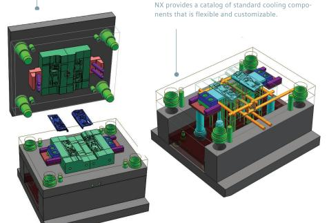
NX accelerates mold manufacturing by documenting the mold design with automated drawing and bill of materials creation.
