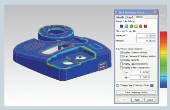
NX validates molded parts by checking wall thickness. Results are displayed in easily interpreted color-coded areas on the part model.
