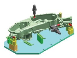
Fixturing designed in NX for a complex part ready for tool paths to be generated in NX Machining.
