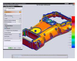
Molded part validation is used to analyze the thickness of part models, providing designers with color-coded visual feedback on the thickness distribution. The information helps designers control cooling rates and part quality. Three-dimensional annotation can be used to document models for downstream processes.
