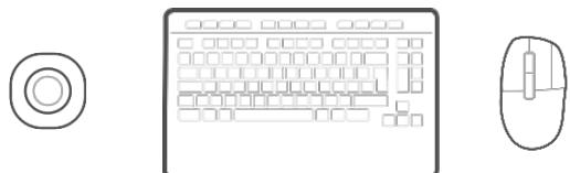
Place the SpaceMouse Wireless on the opposite side of the keyboard to your standard mouse. One hand engages the 3D mouse to position your model: rotating, panning and zooming. The other hand uses the standard mouse to select, create and edit.
