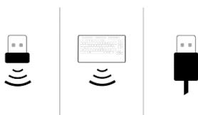
The SpaceMouse Wireless can be connected via the included 3Dconnexion Universal Receiver, the 3Dconnexion Keyboard Pro, or USB cable.
