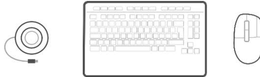
Place the SpaceMouse Compact on the opposite side of the keyboard to your standard mouse. One hand engages the 3D mouse to position your model: rotating, panning and zooming. The other hand uses the standard mouse to select, create and edit.
