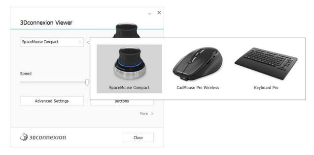
If multiple 3D connexion devices are connected, you can select the desired product to configure by clicking on the flyout button at the top left of the panel.
