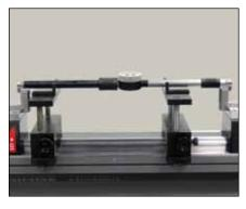
Setting of 2-point internal and external comparative measuring equipment (TEL5/TELMA7/TELMN7.2)
