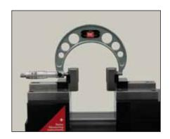
Checking of external micrometers (TEL5/TEL11)
