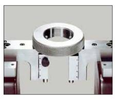
HPA: Checking of thread ring gauges (TEL18)
