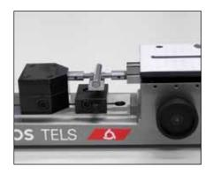
Checking of external diameters (TELS50, TELS5, TELS5.1)
