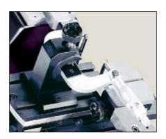
Checking of external micrometers (HPA-1/TULM14)
