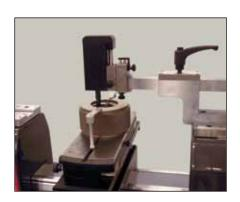
HPD: Checking of thread ring gauges (TA-SU-313/LABC-70/TA-SU-354)
