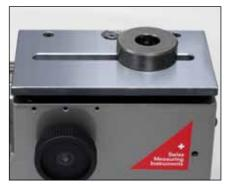
Checking of internal diameters (TELS10)
