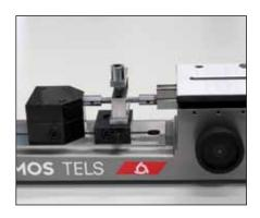
Checking of lengths (TELS50, TELS5, TELS5.1)
