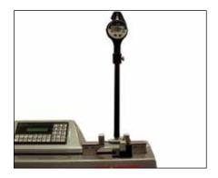
Setting of two-point bore gauges
