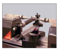
Checking of thread plug gauges (HPA-1/TEL6/3P/0.17-3.2/S6.5/LABC-15)
