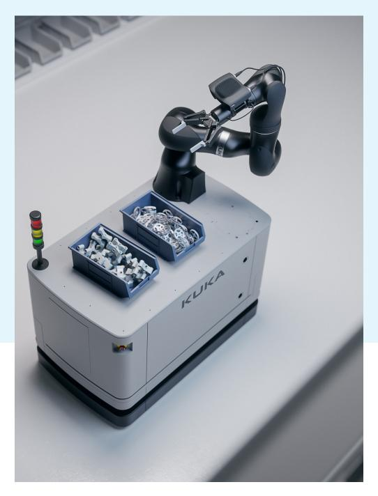
Random bin picking is typically at the input stage of a manufacturing process. Instead of traditional static fixtures or pre-filled stacking patterns, a robot is instead emptying a bin bulk-filled with parts for placing on, for example, a feeder, conveyor, or sorter for further processing in the plant. The choice of the vision system and, in particular, the 3D camera impacts the robot's ability to successfully detect, pick, and place all types of parts.
