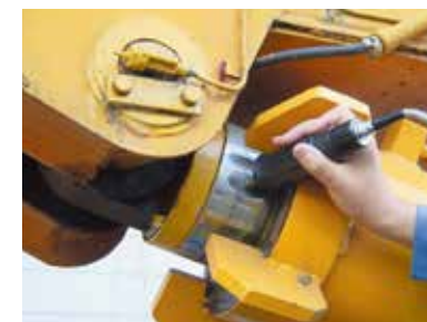
● Diagnosing wear and tear using hardness measurements
