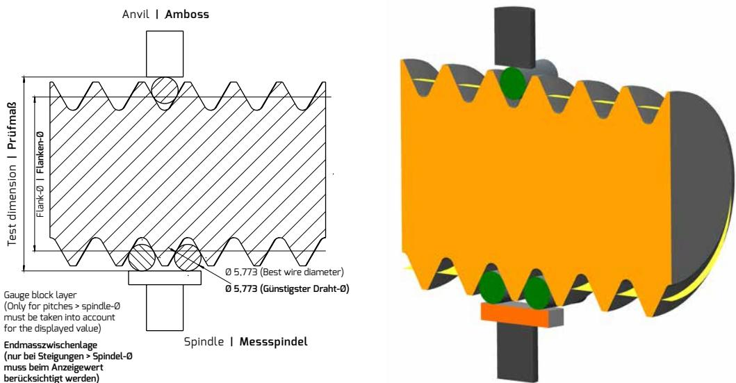
purpose, it is necessary that a specific measuring wire diameter is used for each thread, i.e. the „most beneficial measuring wire diameter“.
