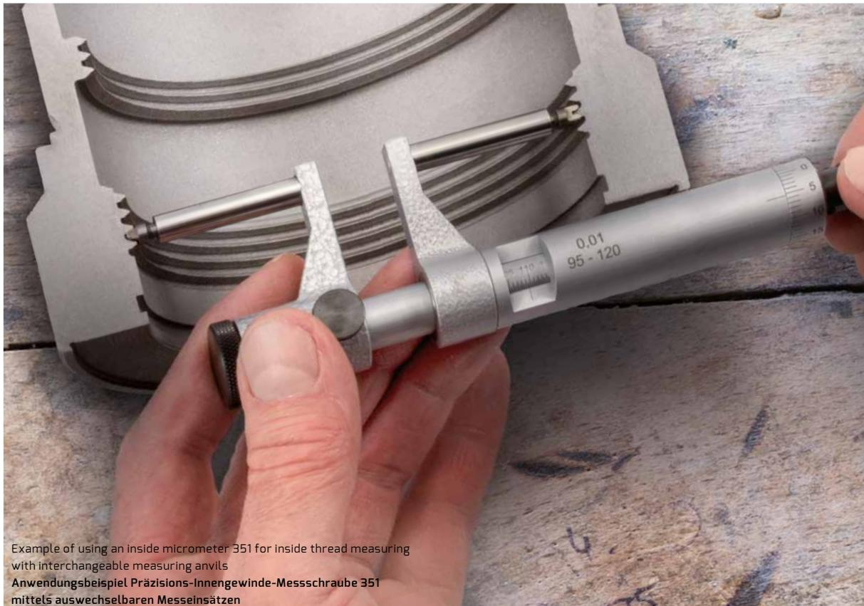
Example of using an inside micrometer 351 for inside thread measuring with interchangeable measuring anvils
