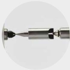
FOR SETTING EXTERNAL THREAD MICROMETERS
