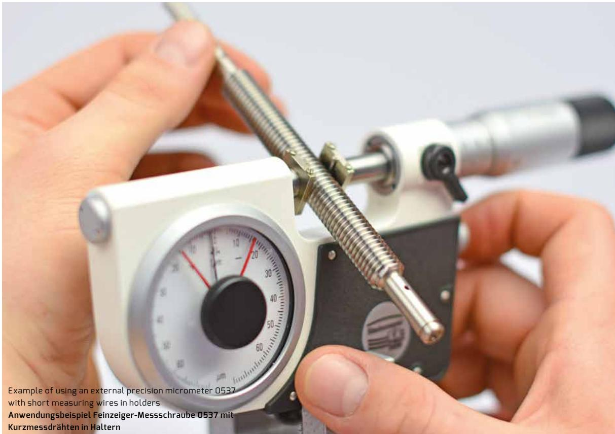
Example of using an external precision micrometer 0537 with short measuring wires in holders
