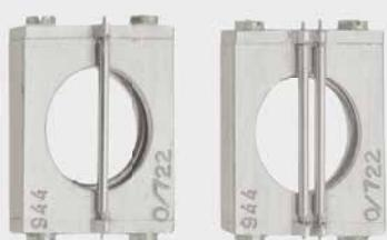
TO MEASURE THE PITCH DIAMETER ON EXTERNAL THREADS USING THE THREE WIRE MEASURING METHOD WITH EXTERNAL MICROMETERS OR LINEAR MEASURING TOOLS.
