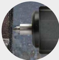
FOR CHANGE MEASUREMENTS OF THE CRANK WEBSPACING OF THE BUILT-IN-ROTATING CRANKSHAFTS AS A MEASURE FOR THE ALIGNMENT OF THE BEARINGS
