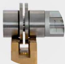
TO MEASURE THE WIDTHS OF KEYWAYS AND KEYSEATS
