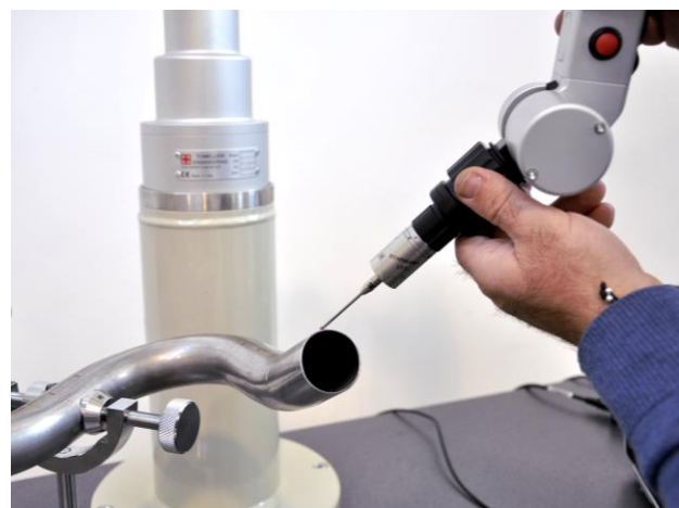
Pipe measurement by touch probe
