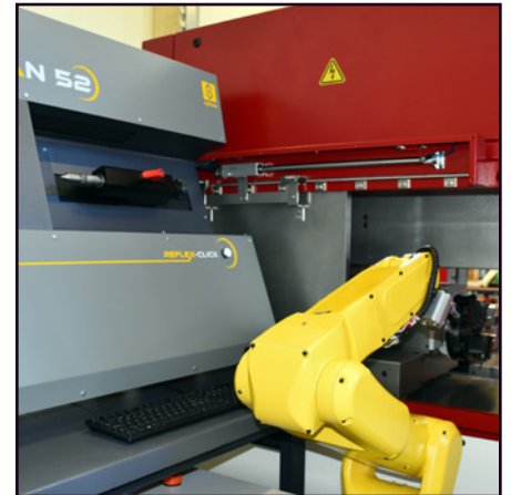
SCAN 52 and robot : closed loop with automatic correction of the part
