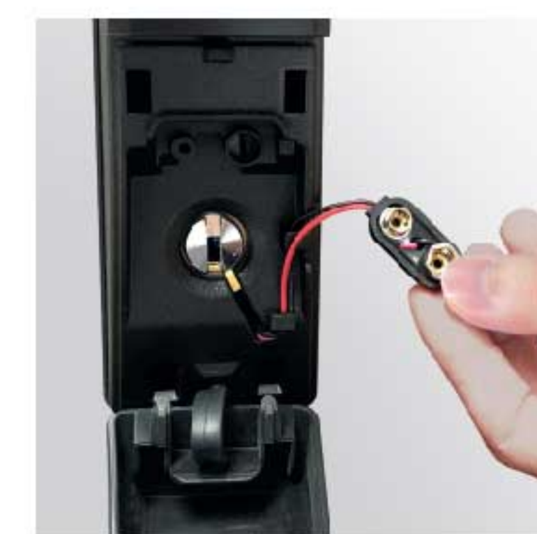
Emergency power supply (9 V battery)
