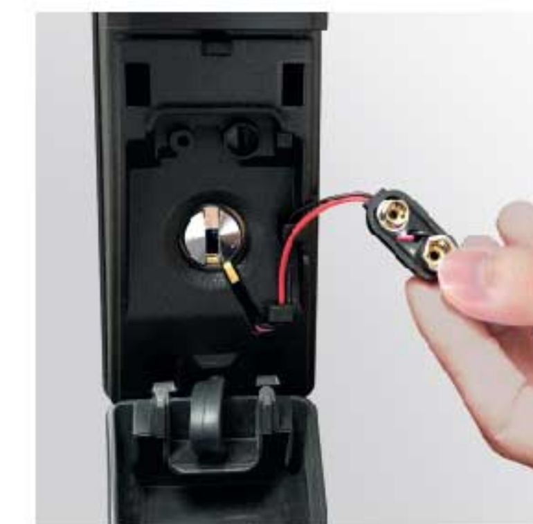
Emergency power supply (9 V battery)
