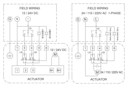
Use proper size of wire and fuse to prevent actuator failure. The data is provided below to assist on the selection of the proper wire and fuse.
