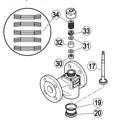
Coat the stuffing box thread with temperatureresistant lubricant.
