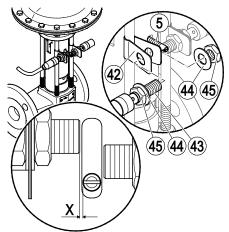
Check the operation of the proximity switch, as described in the manufacturer's installation & operating manual.
