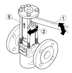
The pressed lever is under spring force.
