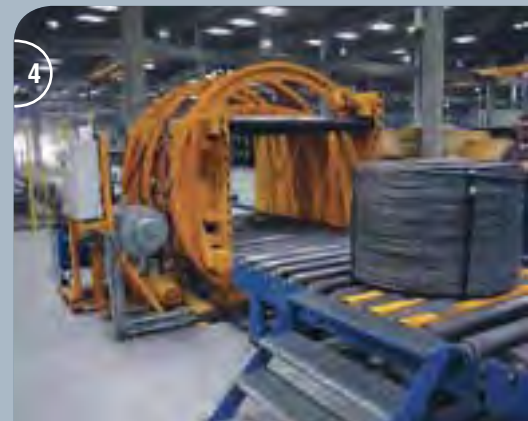
1-4 Elektromotorische Coilwendestation. Electromotive coil turning station.
