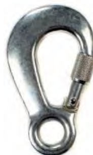
RGK9 EN362 Material - alloy Gate opening – 22mm Size – 108mm x 58mm Closure type – screw gate MBS – 25kN Weight – 157g
