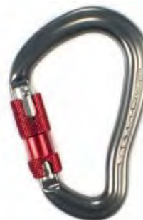
RGK4 EN362 Material - aluminium Gate opening – 25mm Size – 125mm x 90mm Closure type – twist lock MBS – 28kN Weight – 85g
