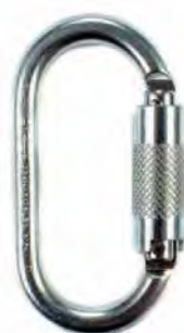
RGK2 EN362 Material - steel Gate opening – 17mm Size – 108mm x 58mm Closure type – twist lock MBS – 25kN Weight – 197g
