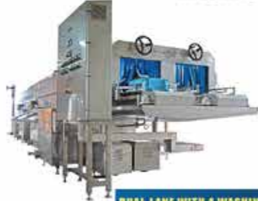
DUAL-LANE WITH 4 WASHING ZONE + BLOW OFF
