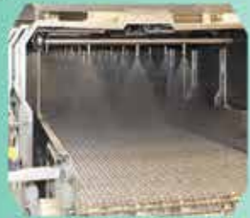
WATER SPRAY COOLING TUNNEL
