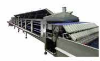
Steam tunnel Cooker
