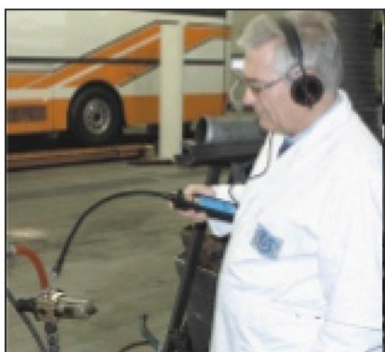
Above shows use of quality headphones and flexible pipe with sensor to get to a difficult spot to find an air leak.
