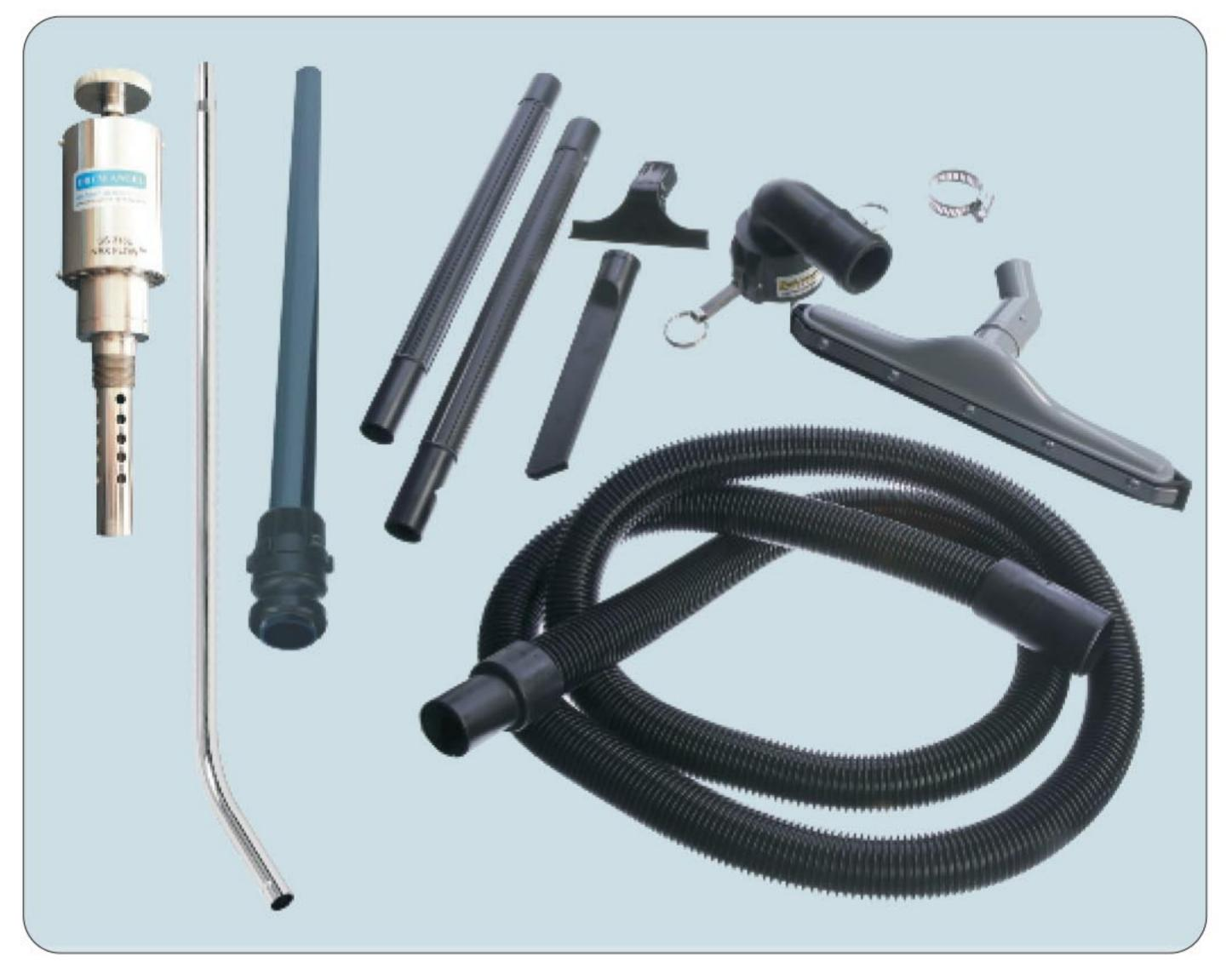
The 316L Stainless Steel Drum Angel Model 35011S includes the Drum Angel unit, crevice tool, skimmer tool and heavy duty squeegee tool, two (2) straight plastic wands, metal wand for use with the heavy duty squeegee tool, 10' of plastic hose with cuffs and drum adaptor with plastic tube. OPTIONAL all 316L stainless drum adaptor and tool available on request at extra cost. Contact representative.
