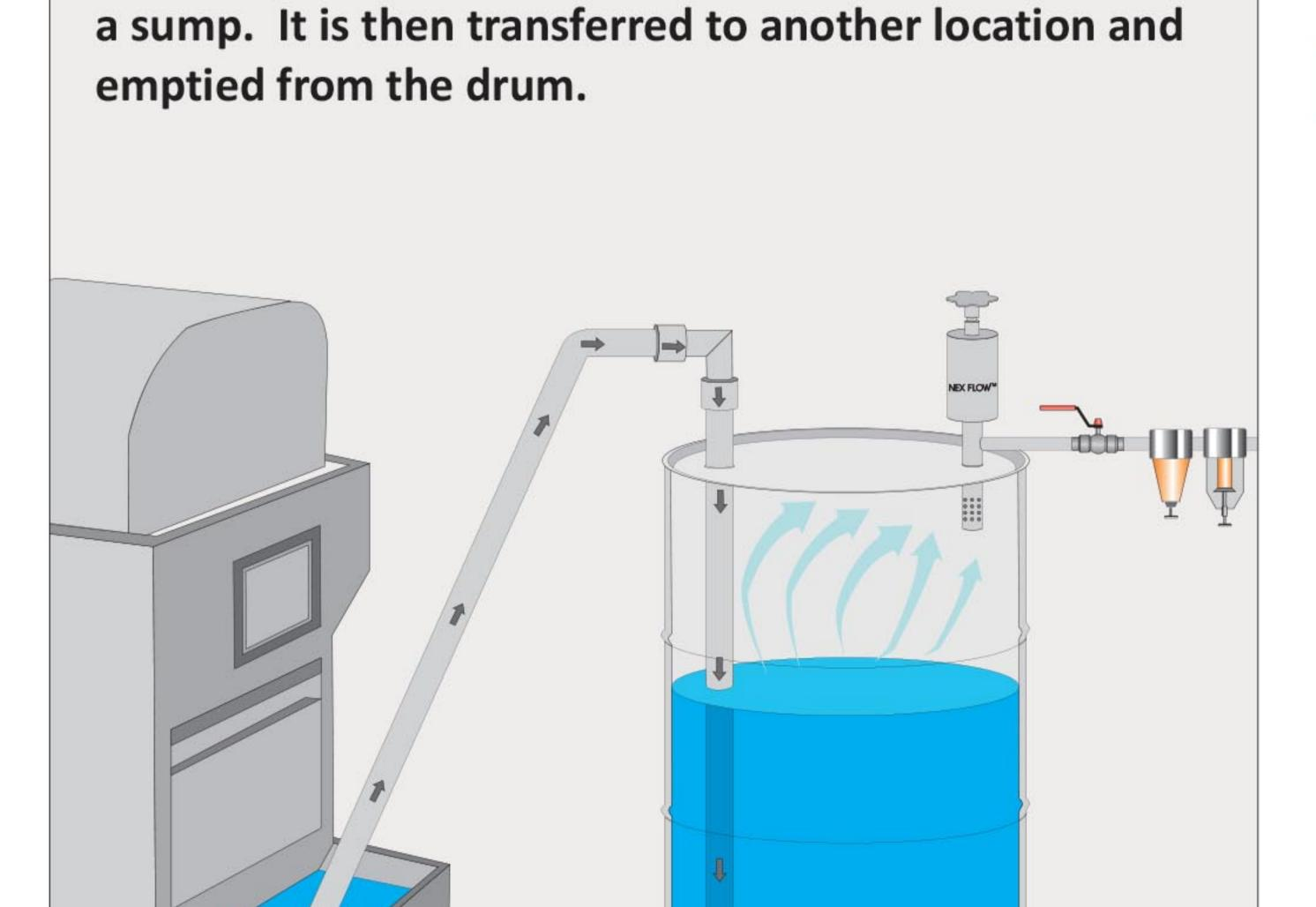
Reversible Drum Angel is used to remove coolant from
