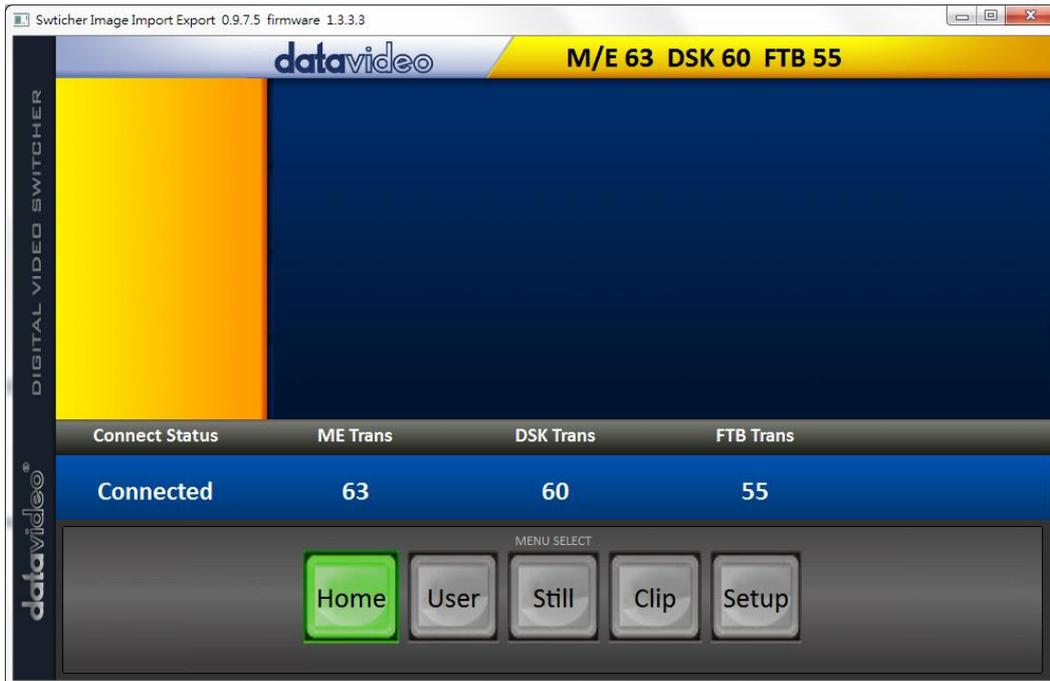
3. After clicking the **Setup** button, the network information will be displayed in the blue area (identical to the SE-1200 MU user control interface).
