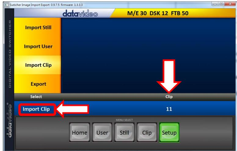
**Note:** The **Switcher Image Import/Export utility** does the conversion from bmp/png/jpg to the .pic file format. All you need is to give the utility a starting file location and it will give the utility an idea where to start linking all images up into a sequential animation file.
