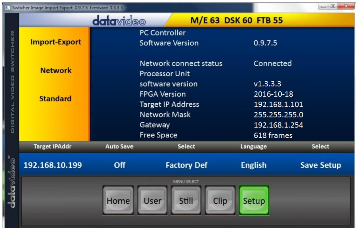
If the network settings are wrong then you may not be able to access the SE-650. Always keep a note of the last IP settings used and change these settings carefully to avoid problems.
