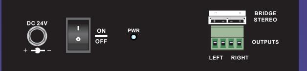
The QTA ACC1 is a high quality compact class D 2×20 watt highly efficient digital amplifier powered by a 24 volt power supply. It can be powered by its own 24V supply or alternatively, by a 24V DC "party line".
