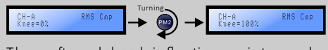
The soft and hard inflection point can be adjusted, among which 0% is the hard inflection point and 100% is the soft inflection point.
