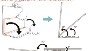
Warning: The rotation range of the hinge is between 0° to 170°. Please do not rotate it more than 170°, otherwise the monitor may be damaged or cracked.
