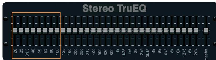
Unlike typical graphic EQs, our **STEREO TruEQ** delivers the exact frequency response for the new fader setting, taking neighboring fader settings into account – for surgical and responsive filtering or general room equalization (Modeled after **BEHRINGER UltraCurve DEQ2496**). The XR16 can provide up to 16 mono graphic EQs – one in each of the 6 Aux Buses and Main LR, plus 8 additional mono GEQ effects (4 stereo) that may be inserted into channels.
