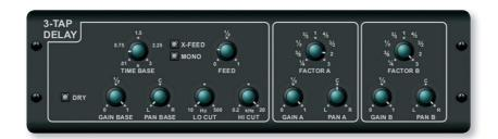
The **3-TAP DELAY** in the X32 RACK records the input signal and then echoes it back after a user-definable period of time and number of repeats. What makes the stereo and triple delay useful and outstanding is the linked tap-timing and musical choice of echo patterns.
