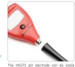
The HI1271 pH electrode can be easily replaced. Just unscrew the electrode from the meter body and screw on a new one.
