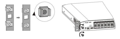
Figure 3-5 Attaching the Brackets to the Rack
