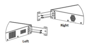
Figure 3-2 Attaching the Mounting Bracket to RG-ES226GC-P
