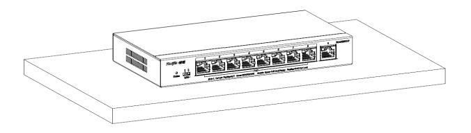
The device must be installed and operated in the place that can restrict its movement.
