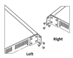
Step 2: Use the supplied M6 screws and cage nuts to securely attach the mounting brackets to the rack, as shown in Figure 3-4 and Figure 3-5.
