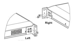
Figure 3-3 Attaching the Mounting Bracket to RG-ES224GC/RG-ES216GC
