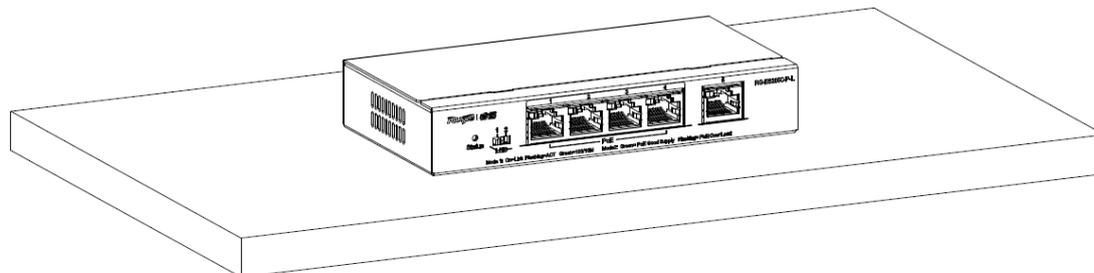
Figure 3-10 Mounting the Switch on the Table
