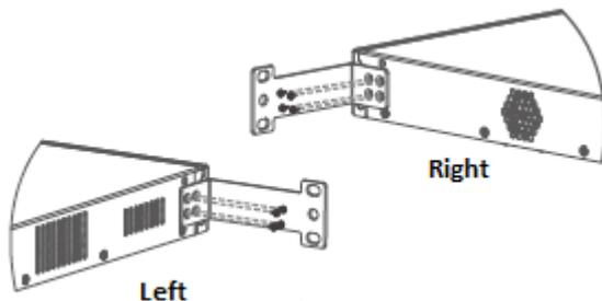
Figure 3-2 Attaching the Mounting Bracket to RG-ES226GC-P
