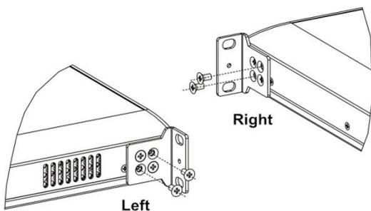
Figure 3-3 Attaching the Mounting Bracket to RG-ES224GC/RG-ES216GC
