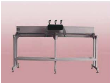
Idler external circular radial run out
