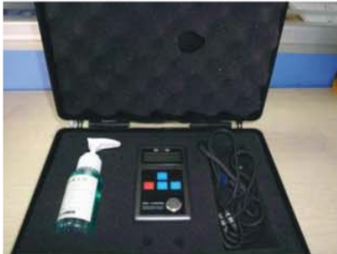
Idler steel tube thickness measuring
