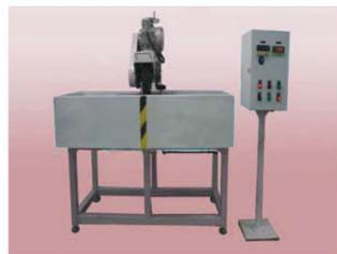
Idler Rotating resistance tester
