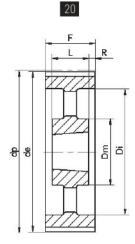
HTD Timing belt pulleys • 14M85 • 14M115
