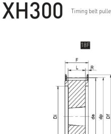
Timing belt pulleys for taper bushes(P.16~P.26)
