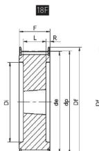
14M55 HTD Timing belt pulleys for taper bushes(P.42~P.52)
