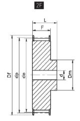
Timing belt pulleys for stock bore(P.1~P.13)
