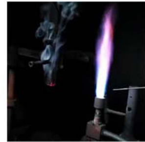
The flame goes out within 10 seconds after leaving the fire
