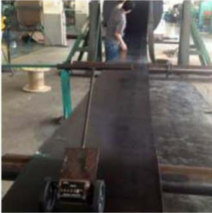
Length and surface inspection
