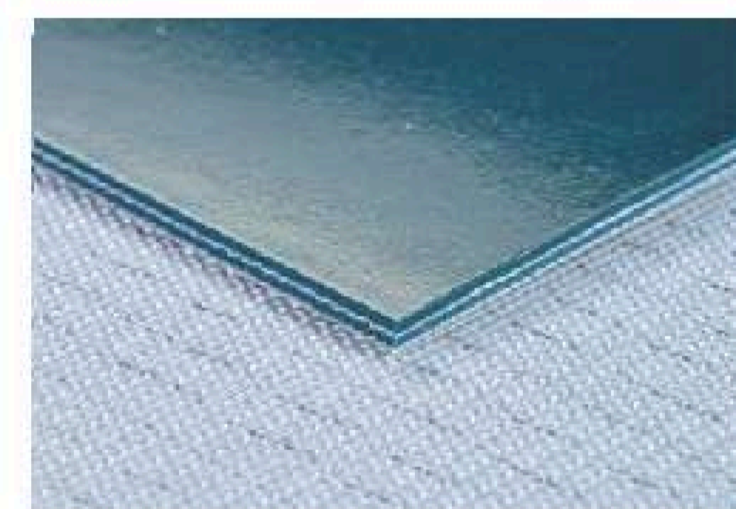
EM120/2:0+1.0/3.0BL/AS HARDNESS*SHA: 80 1% ELONGATION STRENGTH: 8N/mm ROLLER DIAMETER MIN: 55mm
