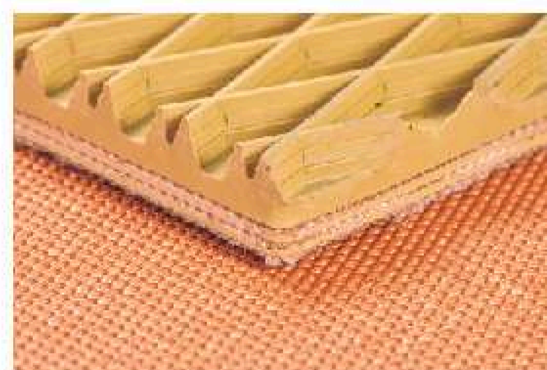
EP200/2:0+5.0RH/7.0TAN HARDNESS°SHA: 65 2% ELONGATION STRENGTH: 16N/MM ROLLER DIAMETER MIN: 80mm
