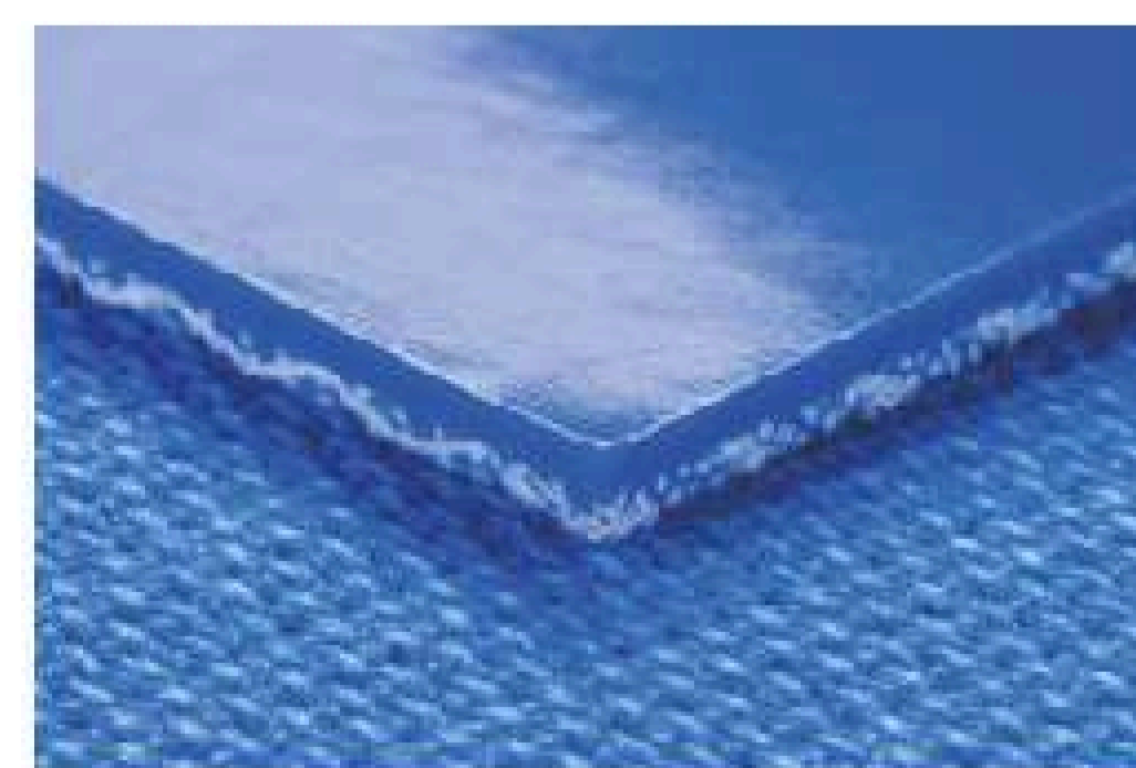
SOLID120/0.1+1.2/3.4SB HARDNESS*SHA: 80 2% ELONGATION STRENGTH: 19N/mm ROLLER DIAMETER MIN: 55mm
