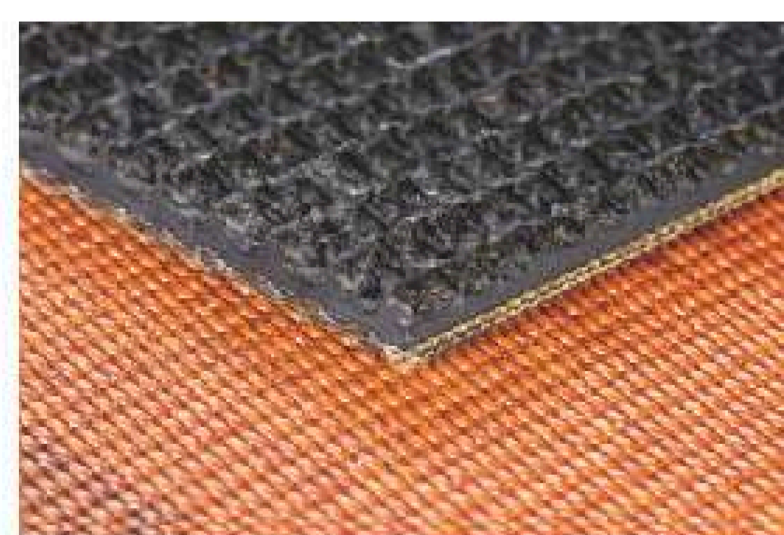
EP200/2:0+4.0SG/6.0B HARDNESS°SHA: 65 2% ELONGATION STRENGTH: 16N/MM ROLLER DIAMETER MIN: 80mm
