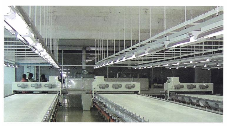
The <u>Infra-red Heated Traveling Carriages</u>, are suitably formatted for applying onto the **Various Types** of **Print Tables**, having being robustly fabricated as a Galvanized Steel **Framework**, supported on adjustable Runner Wheels, and Driven by **AC Inverter Drive** Variable Speed Motor-geared Units.
