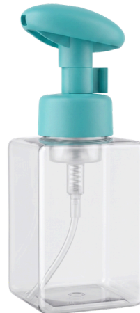
Product Code : CKT-KM-400 Capacity : 400ml. Neck size : 43/410 material : PET weight : 40g.
