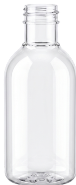
Product Code : CKT-RJ-200-001 Capacity : 200ml. Neck size : 28/410 material : PET weight : 25g.
