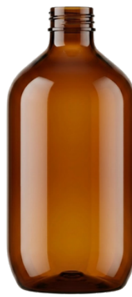
Product Code : CKT-KM-500-004 Capacity : 500ml. Neck size : 28/410 material : PET weight : 30g.
