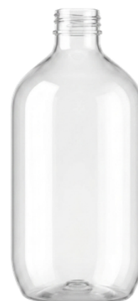
Product Code : CKT-KM-500-006 Capacity : 500ml. Neck size : 28/410 material : PET weight : 30g.
