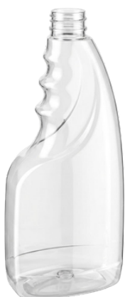
Product Code : CKT-KM-500-005 Capacity : 500ml. Neck size : 28/410 material : PET weight : 40g.
