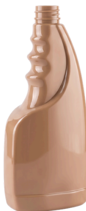
Product Code : CKT-KM-500-003 Capacity : 500ml. Neck size : 28/410 material : PET weight : 40g.
