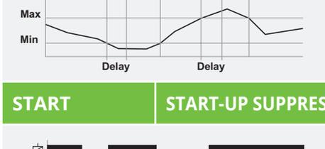
If the monitored value leaves the selected range, the output relay only switches into off-position following expiry of the trip delay.
