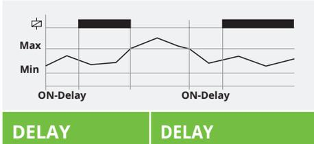
The output relay switches on if the monitored value is within the selected range during the defined time period.
