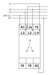
Connected to 1~ 230V mains with power module 230V a.c. without fault latch  $~{\bf I_h}{<}{\bf 10A}$
