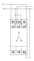
Connected to 3~ 400V mains with power module 400V a.c. and fault latch  $~{\rm I_N}{<}10{\rm A}$
