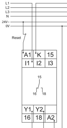
Range 5A with power modul 400V a.c. without fault latch
