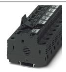
Fuse modular terminal block, fuse type: Glass / ceramics / ..., fuse type: 10:3 x 38 mm, nom. voltage: 1000 V, nominal current: 30 A, connection method: Screw connection, Rated cross section: 16 mm², cross section: 1.5 mm²- 25 mm², mounting type: NS 35/7,5, NS 35/15, color: black
