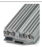
Feed-through terminal block, nom. voltage: 800 V, nominal current: 32 A, number of connections: 4, connection method: Spring-cage connection, 1 level, Rated cross section: 4 mm², cross section: 0.08 mm² - 6 mm², mounting type: NS 35/7,5, NS 35/15, color: gray
