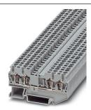
Feed-through terminal block, nom. voltage: 800 V, nominal current: 24 A, number of connections: 4, connection method: Spring-cage connection, 1 level, Rated cross section: 2.5 mm², cross section: 0.08 mm² - 4 mm², mounting type: NS 35/7,5, NS 35/15, color: gray
