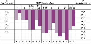
A = A shaded block in the "A" column indicates that the NEMA Enclosure Type exceeds the requirements for the respective IEC 60529, IP First Character Designation. The IP First Character Designation is the protection against access to hazardous parts and solid foreign objects.
