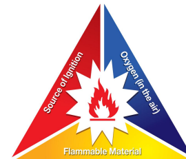
3 - Factors for fire and explosion incident
