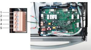
Note: Maximum current drain at the transfer strip: 0.5 A. Only connect external dosing devices with their own fuse protection. Include the dosing device in the protective circuit (PE) of the warewasher.
