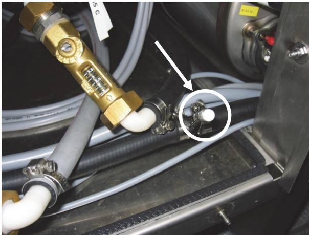
Fig.: Last main wash zone with dosing nipple for rinse aid
