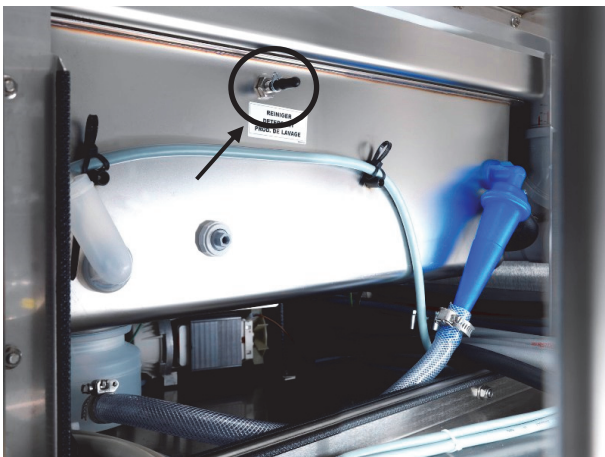
Fig.: First main wash zone with dosing nipple for detergent
