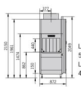
Loading width: 510 mm Loading height: 440 mm
